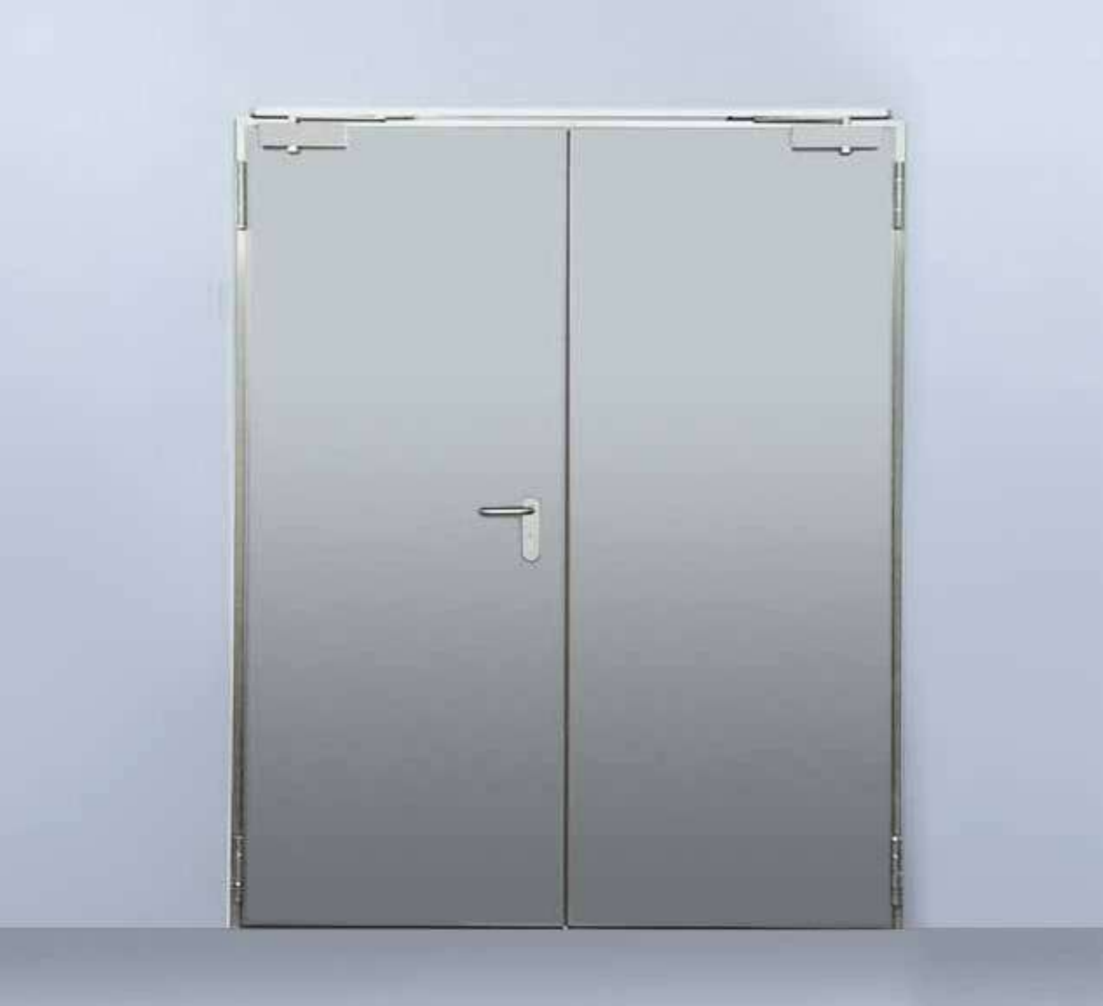
metal collection Art. 11M EI 120 porta a battente 2 ante simmetriche double symmetric fireproof door pannello in metallo preverniciato in colori RAL metal door panel prepainted in RAL colours SP. TH. 8/10 chiudiporta a slitta sequenziale sequential doorcloser cassa in metallo - metal doorframe SP./TH. 15/10 verniciata a polveri RAL - powder coating RAL Mod. PM1WB
