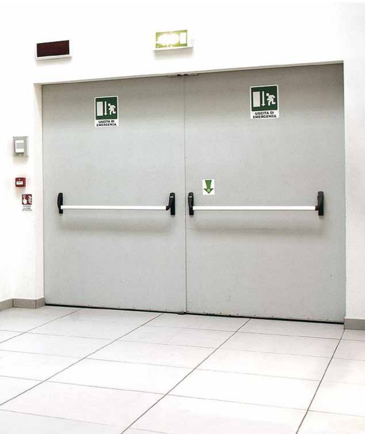
metal collection Art. 11M EI 60 porta a battente 2 ante simmetriche double symmetric fireproof door pannello in metallo preverniciato in colori RAL metal door panel prepainted in RAL colours SP. TH. 8/10 maniglione antipanico a leva panic bar exit device chiudiporta a slitta sequenziale sequential doorcloser cassa in metallo - metal doorframe SP./TH. 15/10 verniciata a polveri RAL - powder coating RAL Mod. PM1TB
