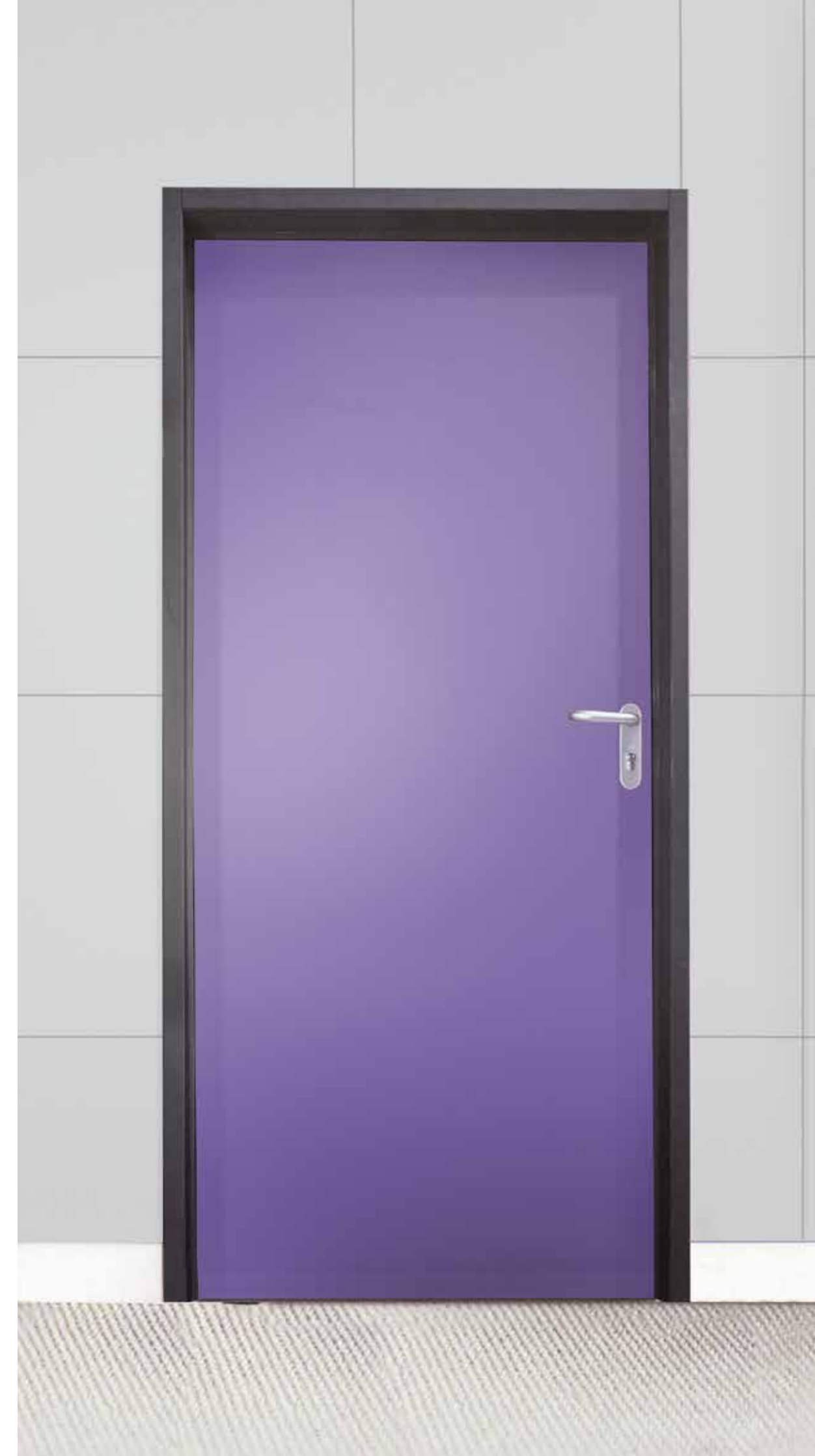
metal collection Art. 11M EI 60 porta a battente - fireproof door pannello in metallo preverniciato in colori RAL metal door panel prepainted in RAL colours SP. TH. 8/10 chiudiporta a molla - spring doorcloser cassa in metallo - metal doorframe SP. TH. 15/10 verniciata a polveri RAL - powder coating RAL Mod. PM1TB
