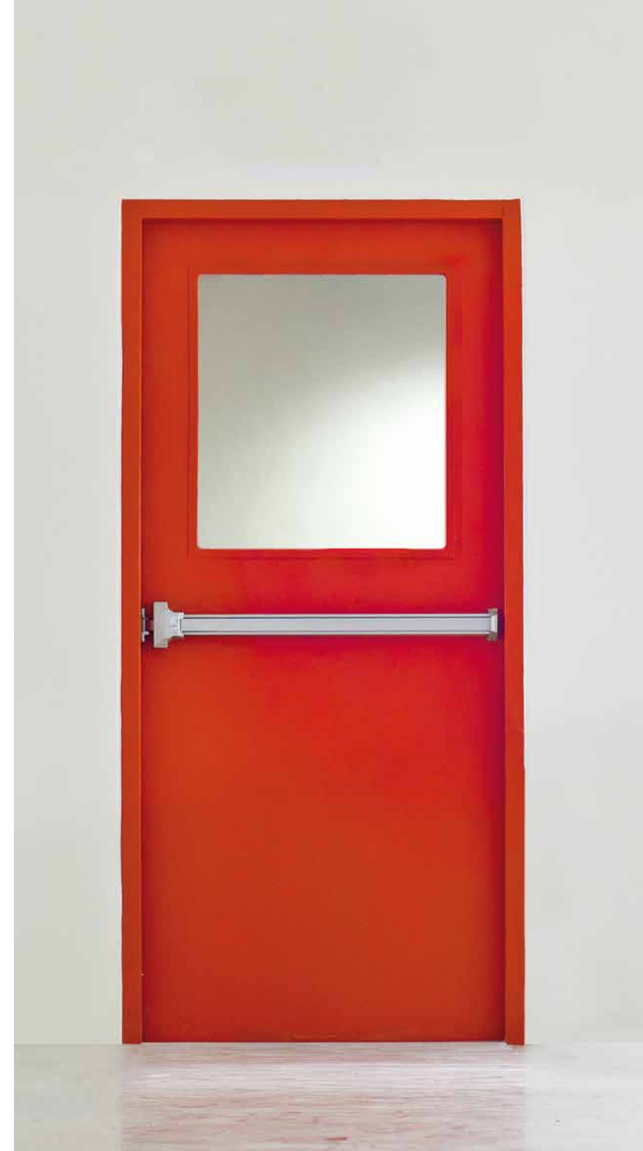
metal collection Art. 11M V6 EI 60 porta a battente - fireproof door pannello in metallo preverniciato in colori RAL metal door panel prepainted in RAL colours SP. TH. 8/10 vetro trasparente - transparent glass Mod. 01A maniglione antipanico push-bar bar panic exit device chiudiporta a molla - spring doorcloser cassa in metallo - metal doorframe SP. TH. 15/10 verniciata a polveri RAL - powder coating RAL Mod. PM1TB
